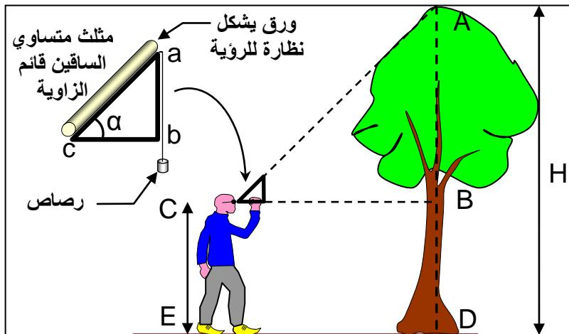
$$\begin{aligned} \text{طول الشجرة} &= AB + BD = AB + CE = AB + BC \\ ? &= AB = CE = BD \\ \text{Tg}\alpha &= AB/BC \Rightarrow AB = \text{tg}\alpha \times BC \\ \alpha = 45^\circ &\Rightarrow \text{tg}\alpha = 1 \\ \Rightarrow AB &= BC \end{aligned}$$
