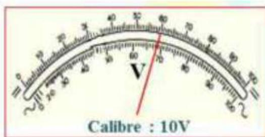
$$\left. \begin{array}{l} C = 10 \text{ V} \\ n = 60 \\ N = 100 \end{array} \right\} \rightarrow \left[ \begin{array}{l} U = \frac{C \times n}{N} = \frac{10 \times 60}{100} \\ \text{Donc, } U = 6 \text{ V} \end{array} \right]$$
