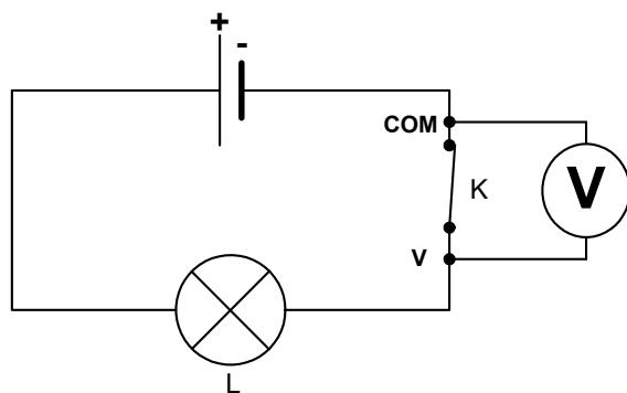
$$U_K = \dots 0 \dots \text{V}$$
