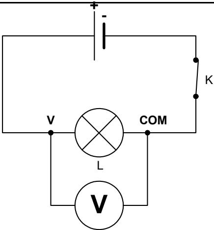
$$U_L = \dots 6 \dots \text{V}$$
