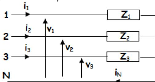
$$I_N = I_1 + I_2 + I_3 = \frac{V_1}{Z_1} + \frac{V_2}{Z_2} + \frac{V_3}{Z_3}$$
