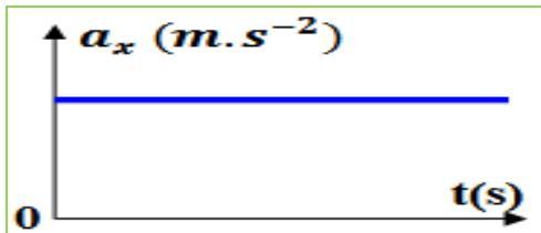
$$\vec{a}_G(t) \left\{ \begin{array}{l} a_x(t) = g \sin \alpha - \frac{f}{m} \\ a_y(t) = 0 \\ a_z(t) = 0 \end{array} \right.$$
