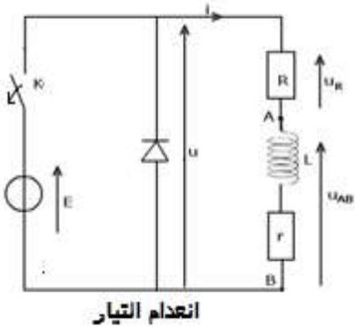
$$u_L(t) = r.i(t) + L \cdot \frac{di}{dt} \quad \text{مع} \quad u(t) = u_L(t) + u_R(t)$$
