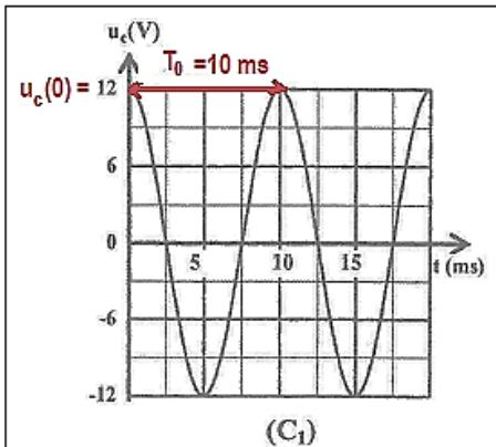
$$T_0 = 2\pi \sqrt{L \cdot C} \Rightarrow T_0^2 = 4\pi^2 L \cdot C \Rightarrow L = \frac{T_0^2}{4\pi^2 C}$$
