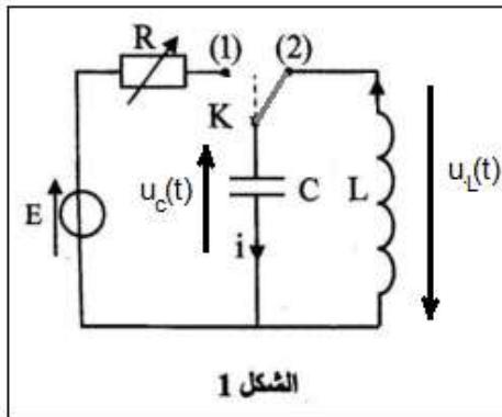
$$\frac{di}{dt} = \frac{d}{dt} \left( \frac{dq}{dt} \right) = \frac{d^2q}{dt^2} \quad i = \frac{dq}{dt} \quad u_L = L \cdot \frac{di}{dt}$$
