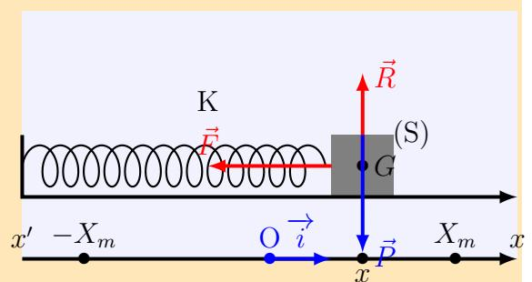
$$\frac{d^2x}{dt^2} = -\frac{4\pi^2}{T_0^2} X_m \cos\left(\frac{2\pi}{T_0 t + \varphi}\right)$$
