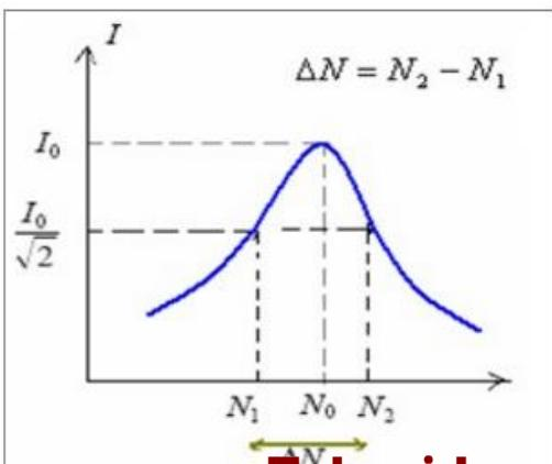
$$P = (R_1 + r_0) \cdot \left( \frac{I_0}{\sqrt{2}} \right)^2 = \frac{1}{2} (R_1 + r_0) \cdot I_0^2$$
