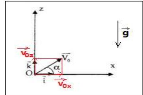
$$\vec{V}_0 \begin{cases} V_{0x} = V_0 \cos \alpha \\ V_{0z} = V_0 \sin \alpha \end{cases}$$
