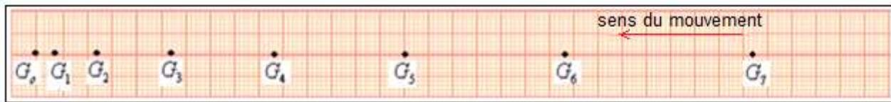
$$G_0G_1 = 3mm, G_1G_2 = 9mm, G_2G_3 = 15mm, G_3G_4 = 21mm, G_4G_5 = 27mm, G_5G_6 = 33mm, G_6G_7 = 39mm$$
