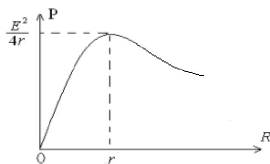
$$\begin{aligned}\frac{dP}{dR} &= \frac{(r+R)^4 - R \times 2.(r+R) \times E^2}{(r+R)^4} \\ &= \frac{r^2 + 2r.R + R^2 - 2.rRr - 2R^2}{(r+R)^4} \times E^2 \\ &= \frac{r^2 - R^2}{(r+R)^4} \times E^2 \\ &= \frac{(r-R).(r+R)}{(r+R)^4} \times E^2 \\ &= \frac{r-R}{(r+R)^3} \times E^2\end{aligned}$$
