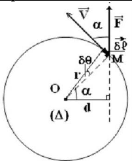
$$P_i = \frac{\delta W(\vec{F})}{\delta t} = \frac{M(\vec{F}_{/\Delta}) \cdot \overline{\delta \theta}}{\delta t} = M(\vec{F}_{/\Delta}) \cdot \frac{\overline{\delta \theta}}{\delta t} = M(\vec{F}_{/\Delta}) \cdot \omega \quad \text{et} \quad \delta W(\vec{F}) = M(\vec{F}_{/\Delta}) \cdot \overline{\delta \theta}$$
